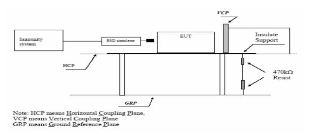
The EUT was put on a 0.8m high wooden tabel/0.1m high for floor standing equipment standing on the ground reference plane(GRP) 3m by 2m in size, made by iron 1.0 mm thick.
