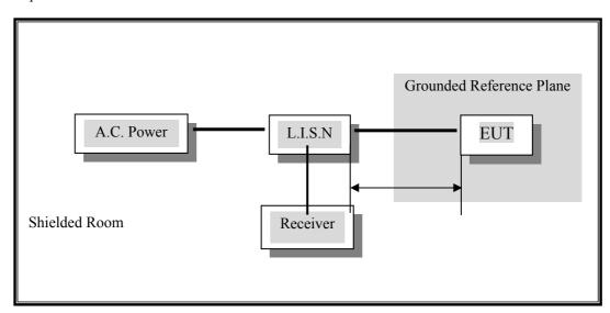
The EUT is on an insulating plane (height=80cm)
